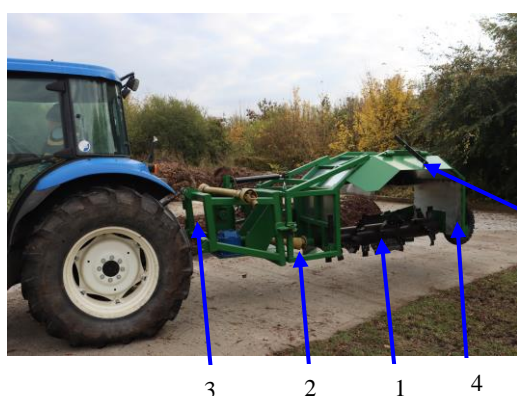
Fig. 1. IAB biohumus loosening equipment [10]: 1 – rotary drum IAB1.0; 2 – support frame IAB2.0; 3– towing support IAB4.0; 4 – side wheel IAB6.0; 5 – steering blade IAB11.0
